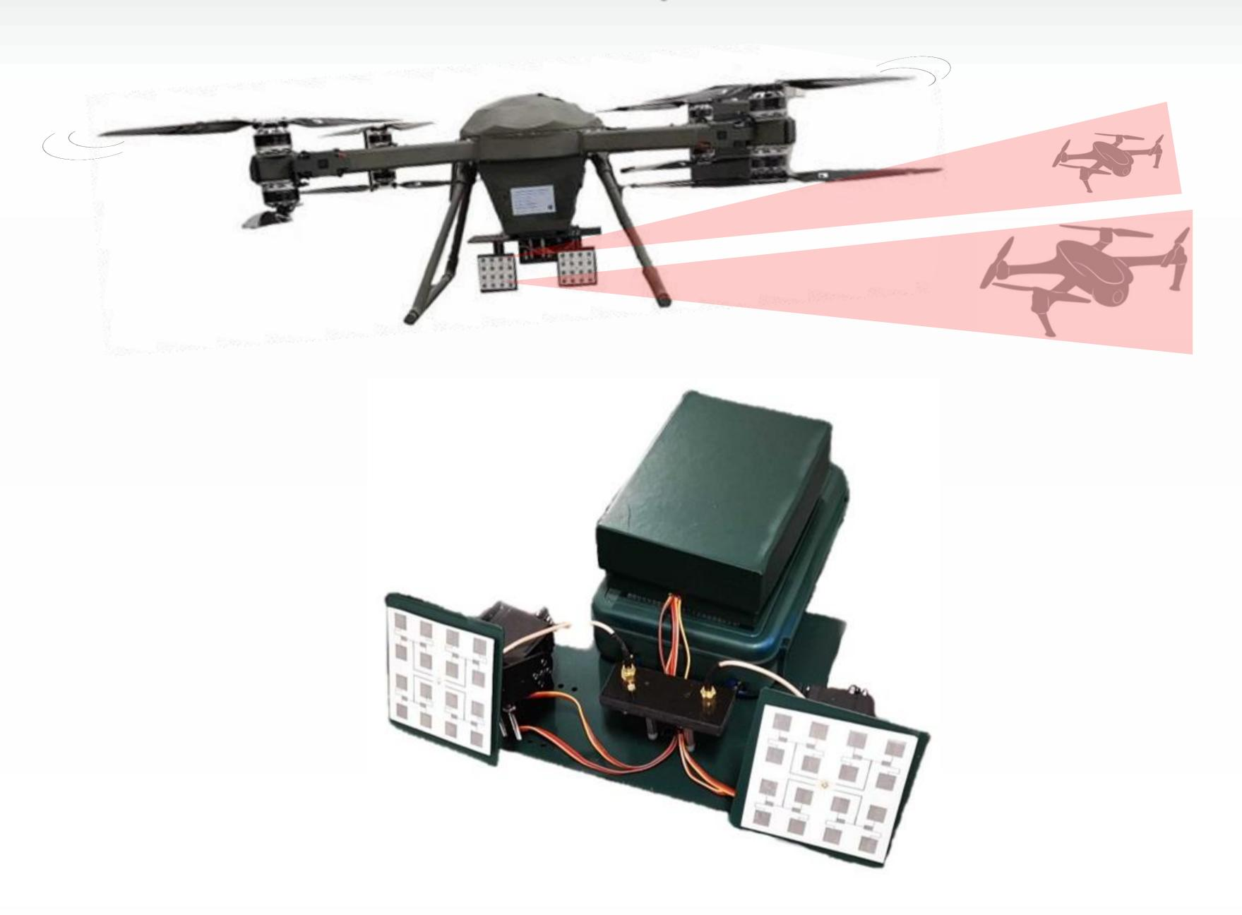
Intelligent Fusion Technology, Inc. has developed the CURADAR, a low SWaP-C radar, that can be mounted on small-sized drones with a small payload. The CURADAR is an excellent counter UAS (unmanned aircraft system), effective in air-to-air detection and tracking of smallsized unmanned aerial vehicles.
