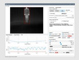
The GUI software for targeting and differentiating detected humans, sensors fusion, while continuously tracking interested human targets.
